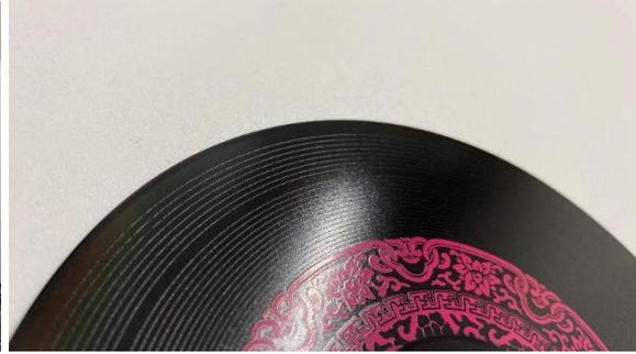
Fig. 6. Laser engraved CD-ROM, as a Bakelite record
